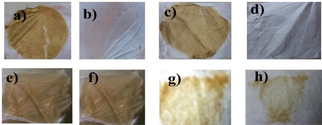
Fig. 2. Back and face layer of cellulose acetate nanofibers (a-f), back and face layer of commercial face mask (g-h)
