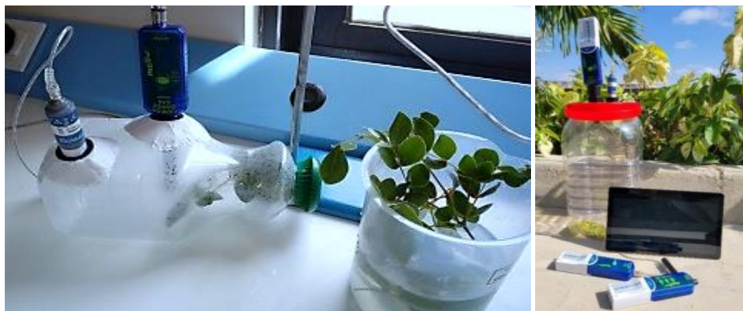
Fig. 1. Leaf Chamber containing CO 2 and O 2 , and Light sensors
