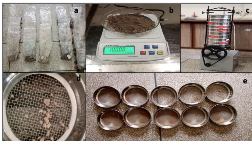
Fig. 2. (a) soil sample bags (b) soil weigh machine (c) sieving instrument (d) sieve showing soil grading (e) set of sieves for soil gradation.
